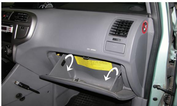
**(EN)** Open the glove locker, open the locks, remove the locker
