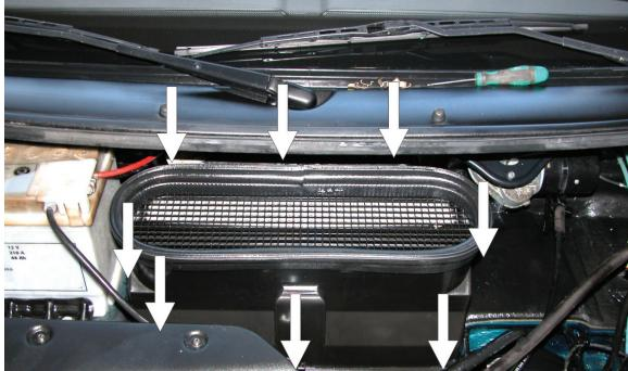
(EN) Unfasten the locks and remove the filter housing
