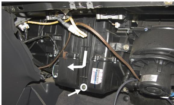
**(EN)** Loosen the screws of the filter housing. Remove the housing
