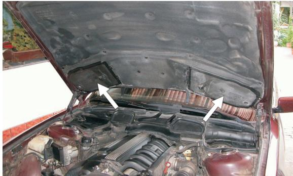
(EN) Open the front bonnet, the pollen filters are located symmetrically on both sides in rectangular housings
