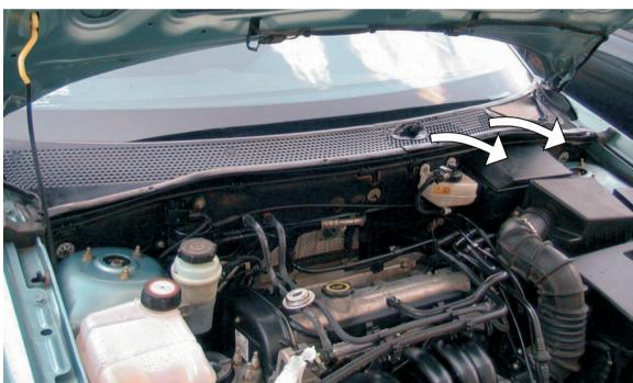
(EN) By lifting it gently disengage first the screen section on the driver's side
