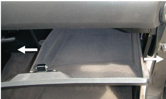
(EN) Open the glove locker, remove the protection of the straps, release the straps, unlatch the hinge, remove the locker
