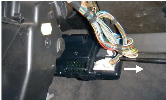
**(EN)** Remove the electronic device located behind the filter chamber
