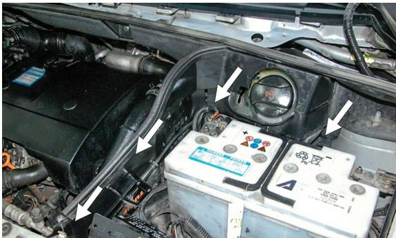
(EN) Remove the partition of the engine chamber
