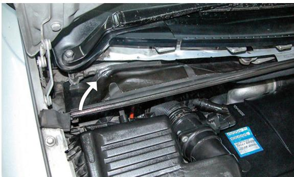
(EN) Remove the rubber seal
