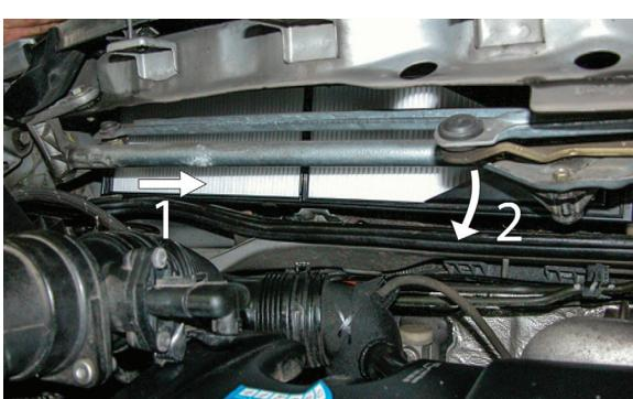
(EN) Gently remove the old filter, put in the new one and carry out the opposite to all the previously mentioned operations in the reversed order
