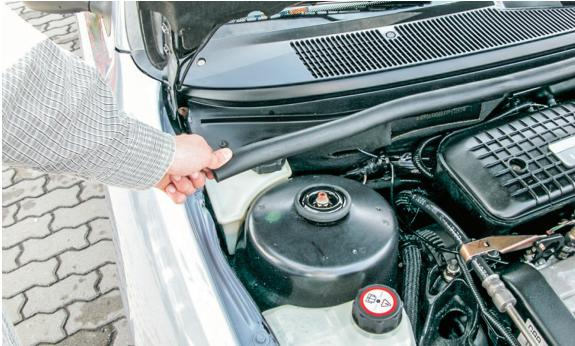
(EN) Remove the rubber seal
