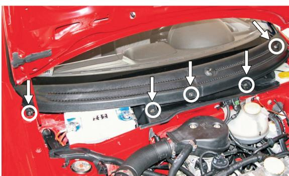
(EN) Loosen the screws of the screen under the windshield
