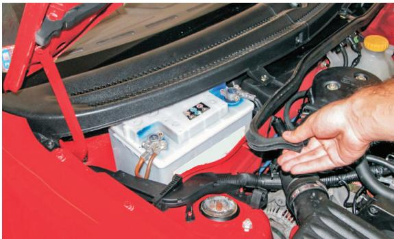
(EN) Remove the rubber seal
