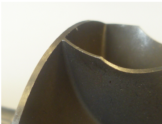
New, undamaged exhaust turbine.
