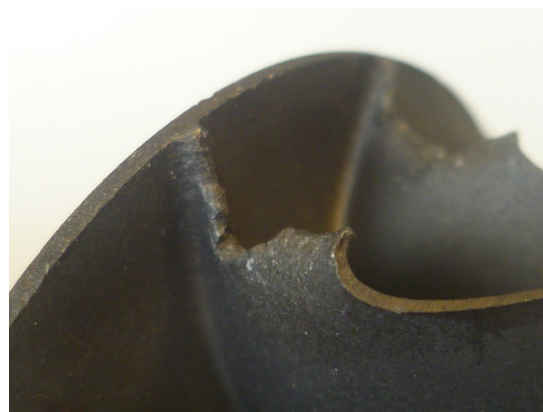
Damaged exhaust turbine.
